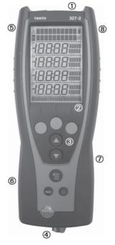
① Head: IR interface (327-2: IRDA) for connection to Testo protocol printers, ON/ OFF switch (①), condensate outlet.
