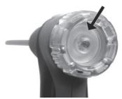
> Check the particle filter of the flue gas probe for contamination at regular intervals: check visually by looking through the window of the filter chamber. Replace the filter if there are signs of contamination. > Replacing the particle filter:
