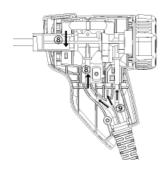
6 Connect adaptor and hose to thermocouple (®). Adjust lines and hoses (③) and attach halfshells.
